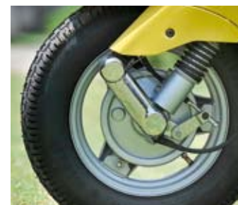
LX125 front drum brake lacks power.
